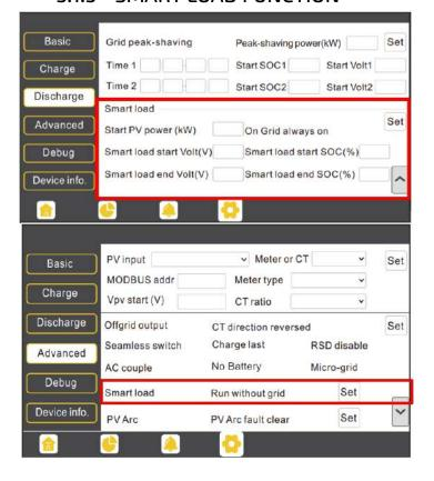
Smart Load: This function will make the GEN input connection point to a load connection point. If enabled, the inverter will supply power to this load when the battery SOC and PV power are above user set values.
