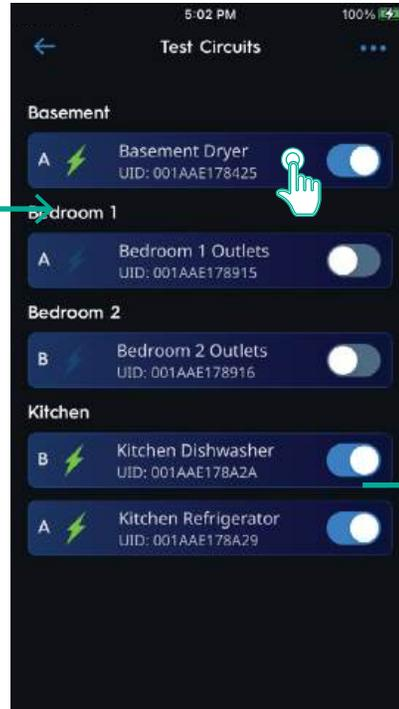
2 TAP CIRCUIT SWITCH TO TOGGLE CHANNEL CIRCUIT ON OR OFF
