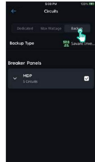
5 TAP BACKUP TO ASSIGN WHICH BREAKER PANEL IS BACKED UP BY THE POWER SOURCE
